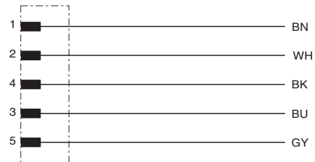
Contact assignment of the M12 plug
